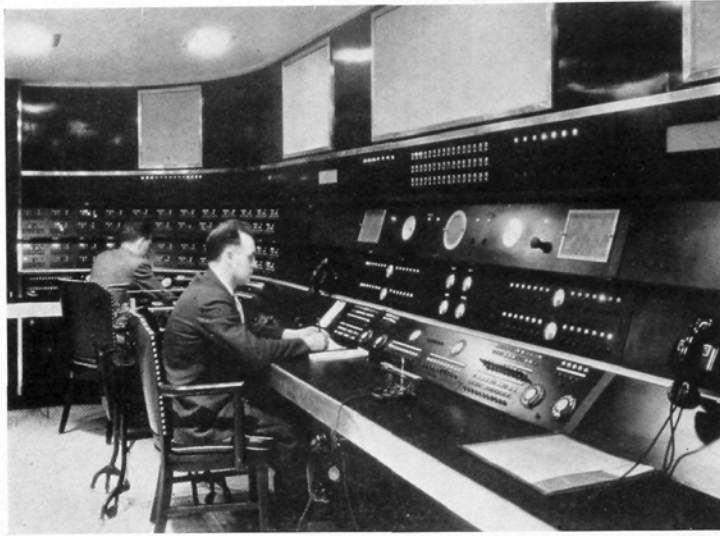
MASTER CONTROL DESK, NERVE CENTER OF BROADCASTING IN THE RCA BUILDING, RADIO CITY
